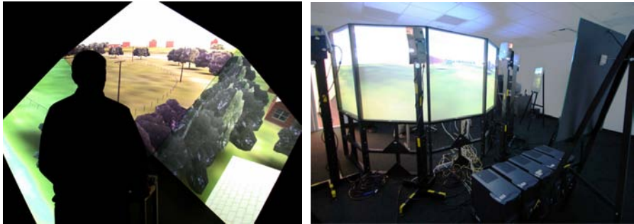
Fig. 2. On the left is a view of an early three facet prototype system in operation. On the right is a rear view of an operational five screen immersive system showing the backside of the display screens, projectors, computers and optical path folding mirrors.
