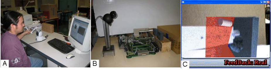
Fig. 3. The different components of the setup. A: The master device. B: the distant haptic robot. C: The VR simulation.
