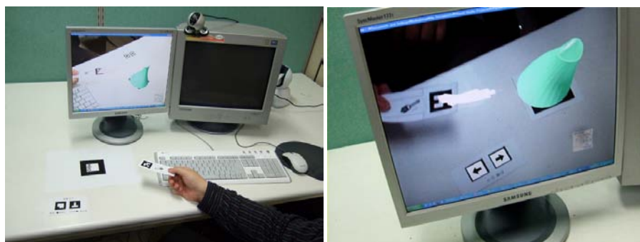
Fig. 1. AR pottery system: the set-up (left), close up view of the display (right)
