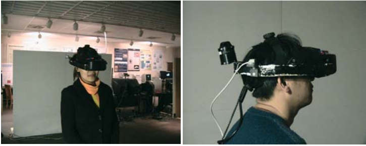
Fig. 4. Head-mounted display system: head-mounted display with head sensor
